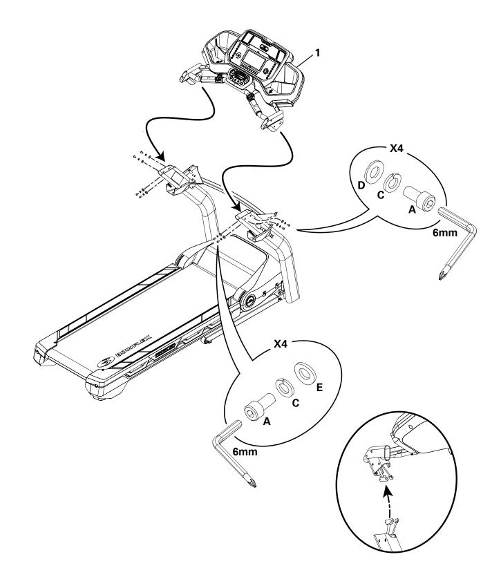
5. Fully Tighten All Hardware from Previous Steps Note: Do not crimp the Cables.
